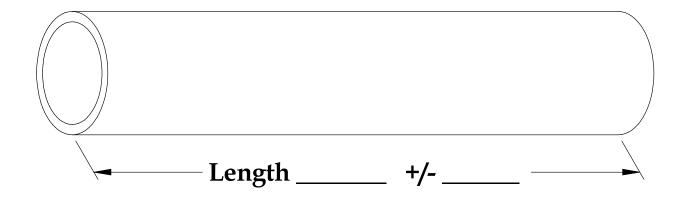
Minimum of two dimensions required below (ID, Wall, OD)
